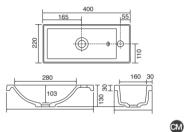
White. Cast Marble. One tap hole. External Overflow. Reversible left/right basin positioning. Suitable for the 400 slimline base/basin units only. Supplied with Chrome overflow ring, see more Type 1 overflow rings on page 333.
