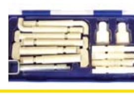
Cover Lifting Set Manhole Cover lifting set with carbon steel zinc plated interchangeable tips. Includes: 2 x 440mm Handles, interchangeable 33mm rectangular Tips, 22mm rectangular Tips, 10mm Side Entry tips, M10 Screw Tips, M12 Screw Tips, M16 Screw Adaptors. 1 Short Stopcock Tip, 1 Long Stopcock Tip. Tips in a small plastic box. ( Spare Nylon Tips 1021T )
