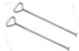
T-End Manhole Cover Keys Heavy duty zinc plated manhole cover lifting keys with rectangular shaped end (lug) and triangular handle. Nominal size of lug 33 x 16 x 5mm ( MLK20 500mm / MLK24 600mm ).
