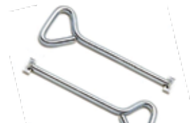
T-End Manhole Cover Keys Heavy duty zinc plated manhole cover lifting keys with rectangular shaped end (lug), triangular handle. Nominal size of lug 33 x 16 x 5mm ( MLK06 150mm / MLK12 300mm ).
